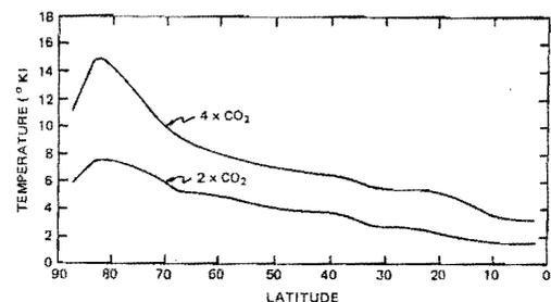
Fig. 2 Surface temperature as a function of latitude after an increase of atmospheric CO<sub>2</sub> content by a factor 2 or 4 (Model Manabe-Wetherald 1980; L. Gates in Bach 1980).
