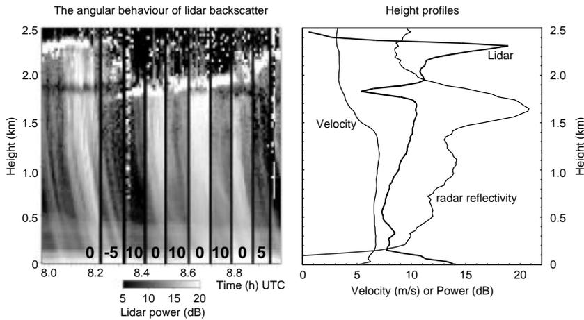
**Figure 2.** The lidar backscatter (Vaisala CT-75K) in the rain as a function of the pointing angle (2a). The angle in degrees is indicated by the big number at the bottom (zenith = 0). The dark band at 1.8 km and the reflections from the ice crystals above it are obscured in the middle of the measurement by a cloud. Fig. 2b shows the profiles of the lidar backscatter, radar reflectivity (dBZ), and radar velocity (m/s) from the beginning (till 8.2 hrs) of the measurement.
