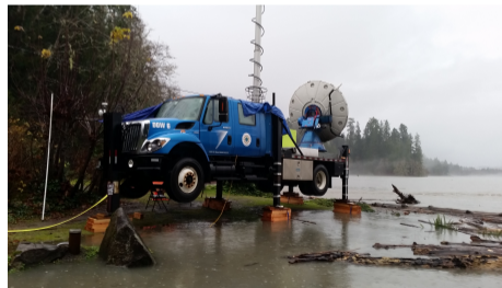
Figure 2: DOW Mobile Radar Instrument during OLYMPEX (University of Washington 2017).
